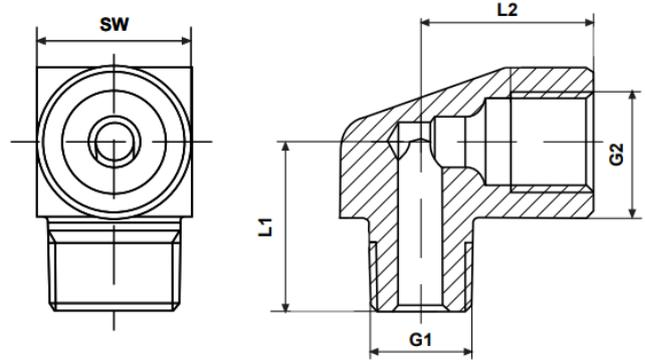
90 degree elbow with conical connection, suitable for 4 mm PA tube.
