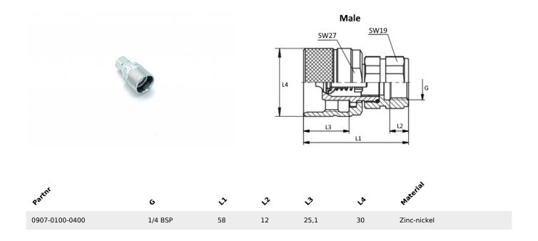
The coupled working pressure is 300 bar
