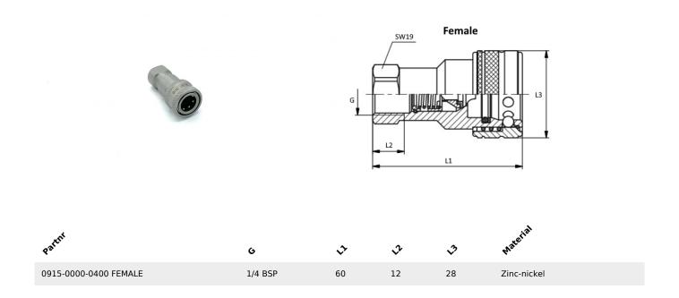
The coupled working pressure is 250 bar
